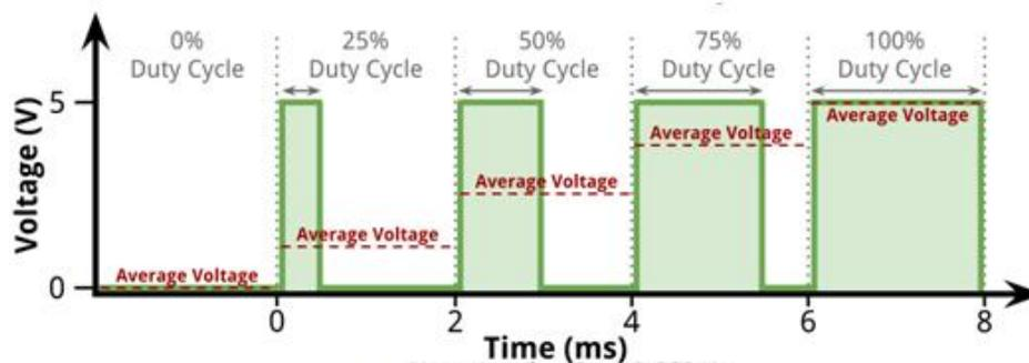
fig.2 Pulse width modulation duty cycle
