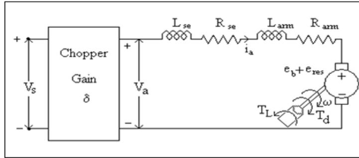
Fig.1 Chopper Controlled DC Series Motor
