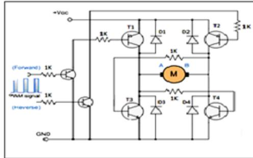
**Fig.2 H-bridge & motor interfacing**
